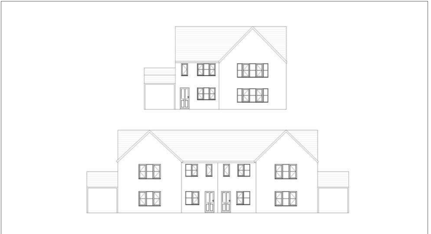
Front elevations of detached and semi-detached properties, from the hypothetical, proposed residential development.
